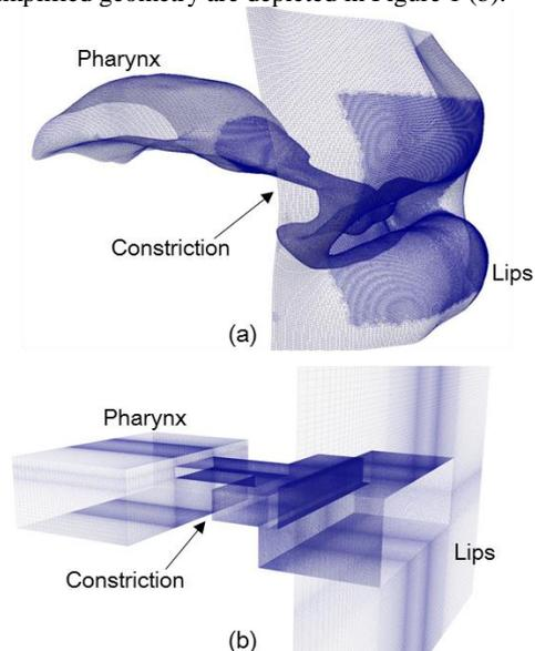
Figure 1: Computational grids of realistic geometry (a) and simplified geometry (b) for the vocal tract of /s/.
